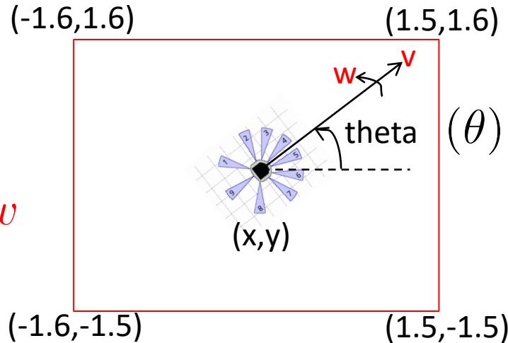
$$\begin{aligned}\frac{dx}{dt} &= v \cos(\theta) \\ \frac{dy}{dt} &= v \sin(\theta) \\ \frac{d\theta}{dt} &= w\end{aligned}$$
