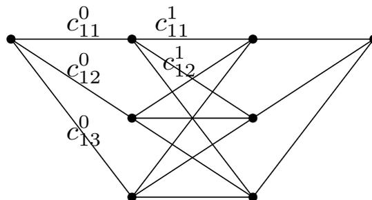
Thus,  $c_{ij}^k$  is the cost from node  $i$  at stage  $k$  to node  $j$  at stage  $k + 1$ . The cost of a path is defined to be the sum of the costs of the links.
