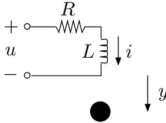
We took the numerical values  $M = 0.1$  Kg,  $R = 15$  ohms,  $L = 0.5$  H,  $K = 0.0001$  Nm<sup>2</sup>/A<sup>2</sup>,  $g = 9.8$  m/s<sup>2</sup>. The problem is to design a controller that will stabilize the ball at  $y = 0.01$  m.
