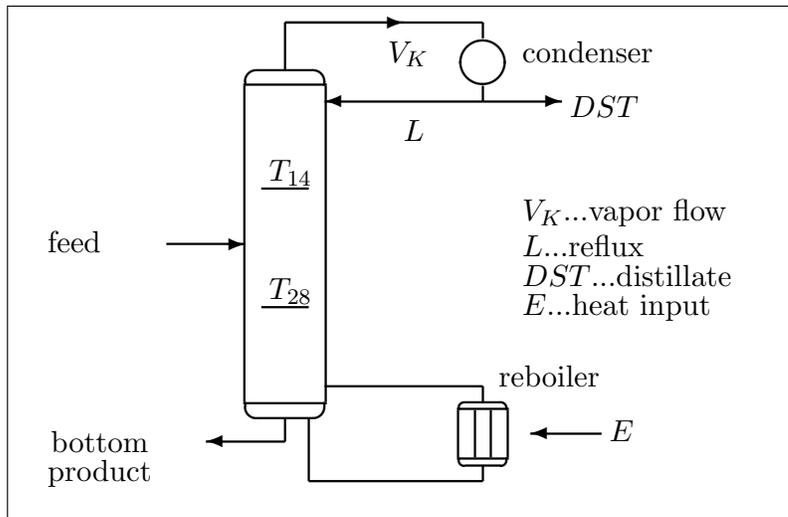
Figure 1: Schematic representation of distillation column
