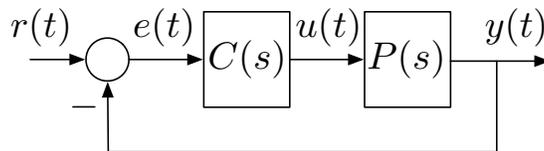
Suppose  $r(t)$  is an arbitrary constant value and we require  $y(t)$  to converge to that constant value. By linearity, it suffices to meet this requirement for just  $r(t) = 1$ . So the problem is: Given  $r(t) = 1$ , design  $C(s)$  to achieve feedback stability and  $\lim_{t \rightarrow \infty} y(t) = 1$ , or equivalently,  $\lim_{t \rightarrow \infty} e(t) = 0$ .
