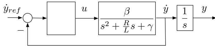
If the loop is well designed, that is,  $\dot{y}_{ref} \approx \dot{y}$ , we can regard the system as merely a kinematic point, with input, velocity, say  $v$ , and output, position,  $y$ .
