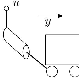
The input is the voltage  $u$  to the motor, the output the cart position  $y$ . We want the model from  $u$  to  $y$ .
