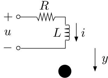
This example was used frequently in ECE356. Imagine an electromagnet suspending an iron ball. Let the input be the voltage  $u$  and the output the position  $y$  of the ball below the magnet; let  $i$  denote the current in the circuit. Then
