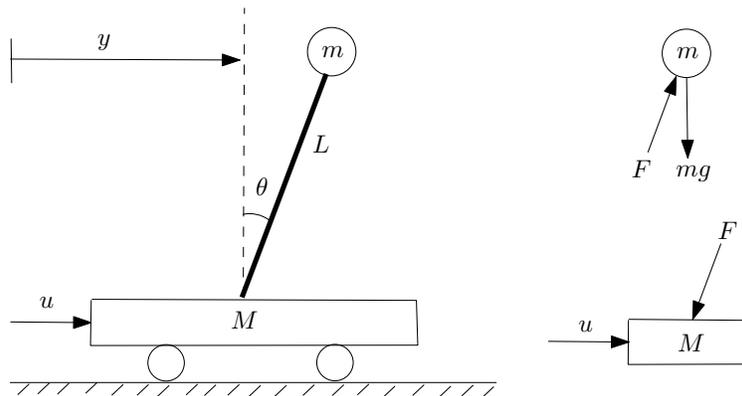
$\theta$ : angle of the pendulum deviated from the upright direction
