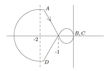
Nyquist plot cannot be drawn by Matlab as a closed contour because Matlab does not indent  $\mathcal{D}$  to the right to avoid pole at s=0
