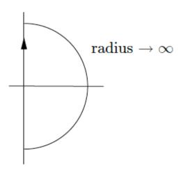
Suppose that G(s) = P(s)C(s) has no poles on the Nyquist contour  $\mathcal{D}$  (indenting to the right if necessary), and has n poles in Re(s) > 0
