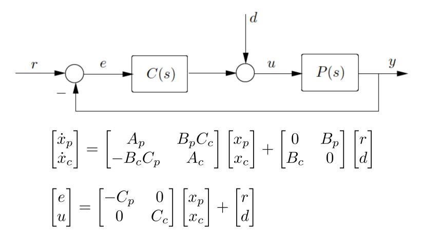
Feedback loop (system) is stable if the eigenvalues of  $A_{cl}$  all have negative real parts
